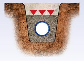
95 % compression (SPO\*) \* SPO : Standard Proctor Optimum Eco- installation using original backfill
