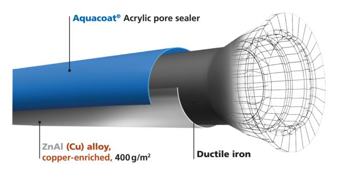
The BioZinalium® coating consists of two layers:
