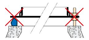
Lay a coat of sealing product around the top of the manhole. The minimum recommended thickness for the coat under the frame, once installed and levelled, is:
