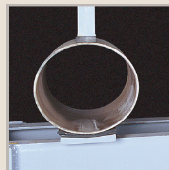
Crushing strength of a GRP tube
